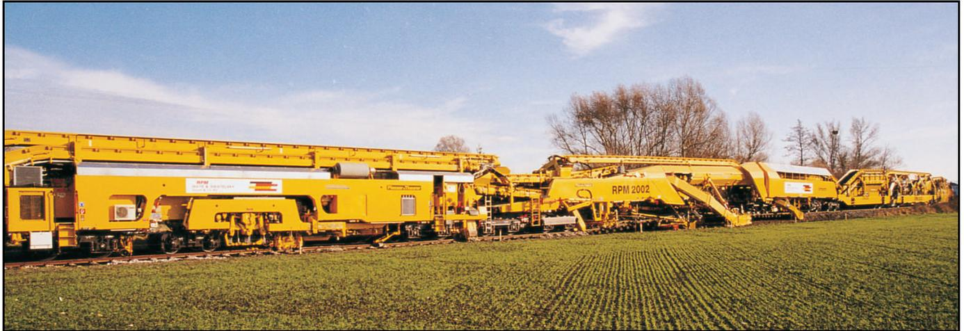
Plasser & Theurer has developed the Millennium Machine, a formation rehabilitation machine with integrated ballast recycling. It is the longest machine the company has ever built.
