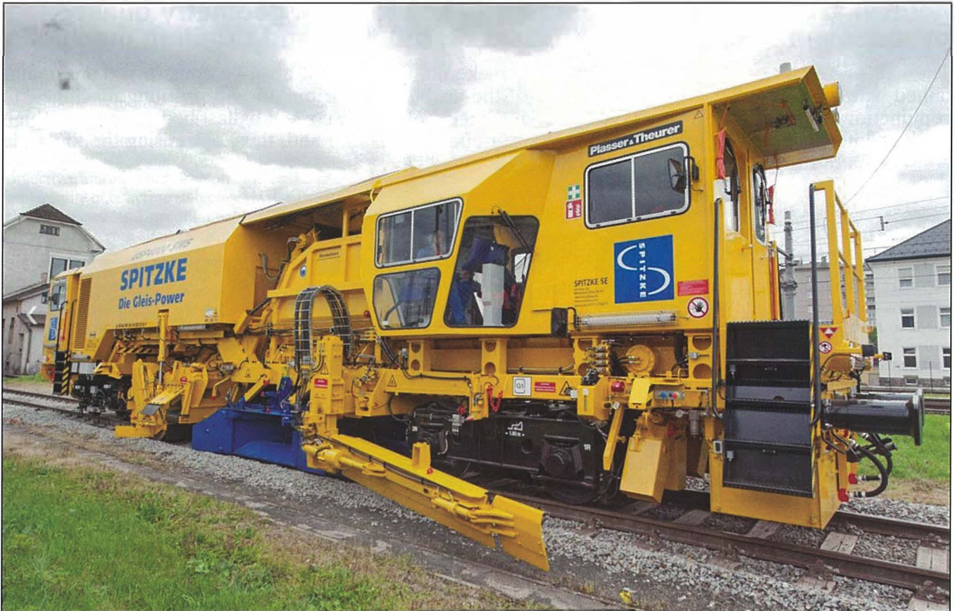
Fig. 2: The Plasser & Theurer USP 4000 SWS ballast distribution and profiling machine for plain track and turnouts — this machine, in conformity with TSI Noise 2015 [2], has a number of noise and dust reduction features, thus making it suitable for operation in areas that are sensitive to noise and dust emissions
