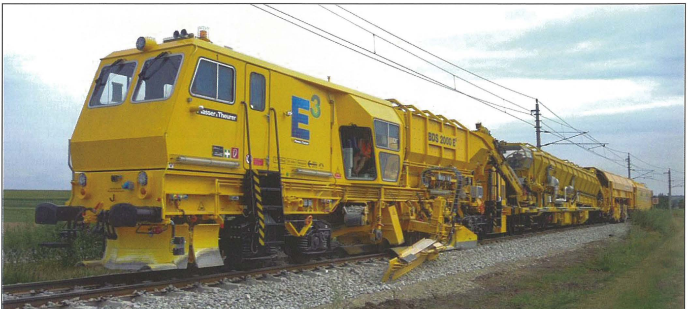
Fig. 1: The Plasser & Theurer BDS 2000 E 3 ballast distribution and profiling machine with hybrid drive technology achieves a high efficiency in ballast management in an environmentally-friendly manner
